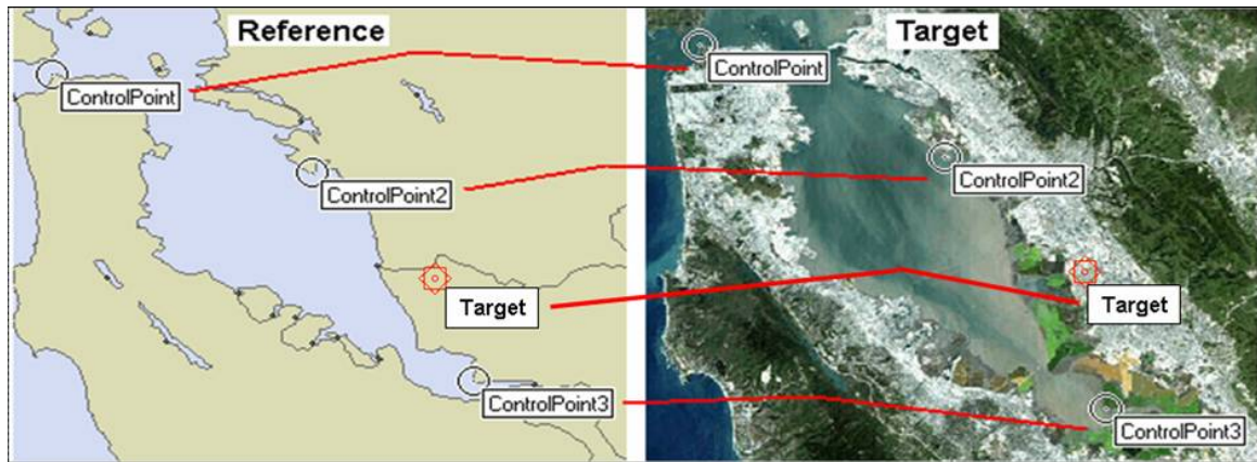
Figure 2.19: Georeferenced control points with unique features are used to georegister a target in a satellite image to a reference map (image provided by Manifold Systems).
